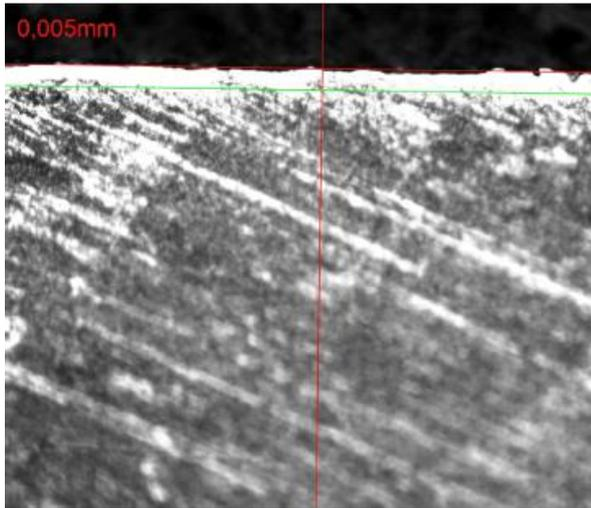
Fig. 3: light optical micrograph of an Expanite-hardened Inconel 718 evidencing a homogenous case-depth in the range of 5-10 $\mu$ m. Surface hardness measurements reveal ca. 1,000 HV0.025
