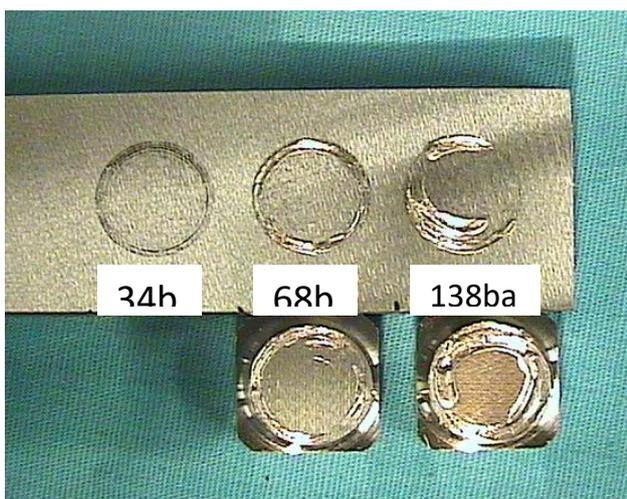
Fig. 1: galling result on non-treated 316-material showing significant galling at relatively low contact-pressure
