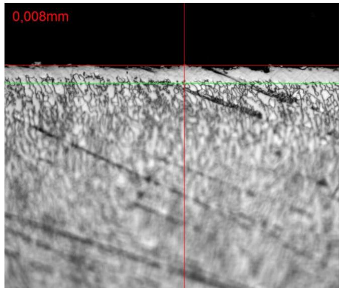
Fig. 4: light optical micrograph of an Expanite-hardened Stellite 1040 showing a hardened zone of ca. 8 $\mu$ m. Surface hardness measurements resulted in ca. 900HV0.025
