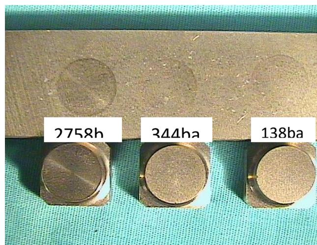
Fig. 2: galling result on Expanite-hardened 316-material showing absolutely no galling even at contact pressures well above yield strength
