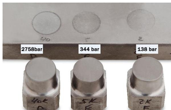
*Fig. 2: galling result on Expanite-hardened 316-material showing absolutely no galling even at contact pressures well above yield strength*
