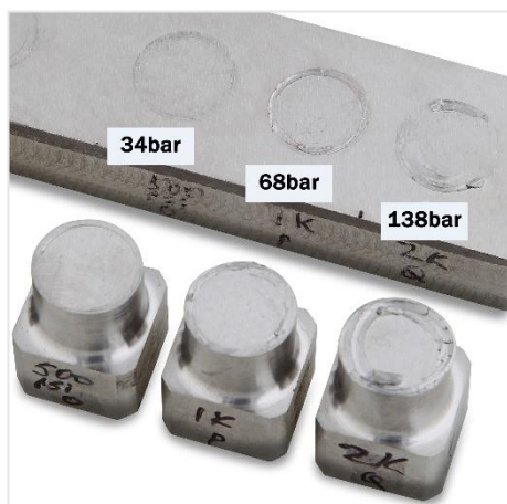
Fig. 1: galling result on non-treated 316-material showing significant galling at relatively low contact-pressure
