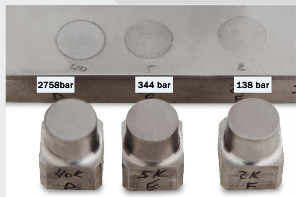
Fig. 2: galling result on Expanite-hardened 316-material showing absolutely no galling even at contact pressures well above yield strength
