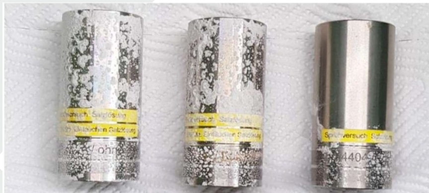
Fig. 7.: Results of the salt spray test on SuperExpanite hardened 316L alloy part (far right) as compared to competitors' solutions.
