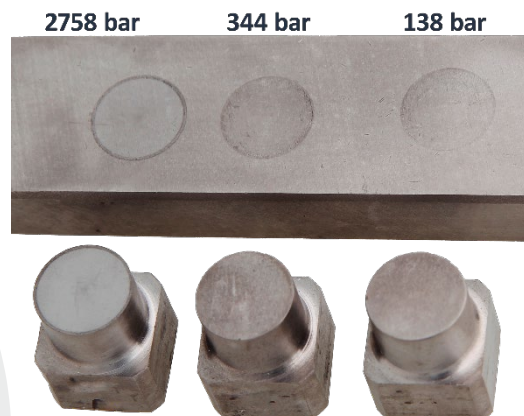
Fig. 6: SuperExpanite treated AISI 316L test specimens after ASTM G98
