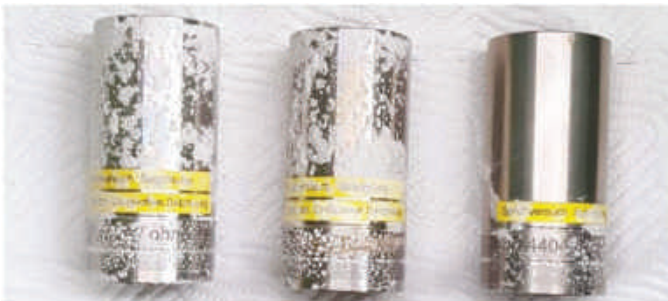
Figure Five: Results of the salt spray test on SuperExpanite® hardened 316L alloy part (far right) as compared to competitors' solutions
