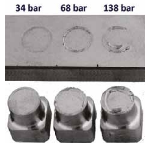
Figure 5. Untreated AISI 316L test specimens after ASTM G98
