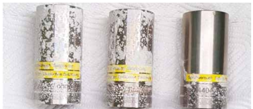
Figure 7. Results of the salt spray test on SuperExpanite hardened 316L alloy part (far right) as compared to competitors' solutions
