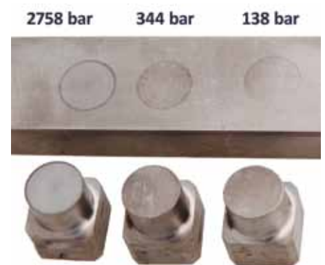
Figure 6. SuperExpanite treated AISI 316L test specimens after ASTM G98
