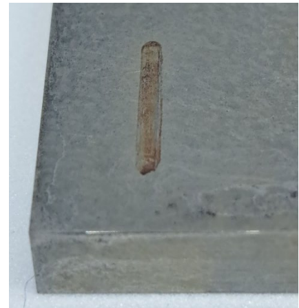
Figure 4: Wear track on the flat test block after ASTM G133 wear test. Alloy 1.4021 treated with SuperExpanite10 (NC Cryo) against 100Cr6 ball bearing.
