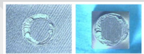
Figure 1: Severe galling of untreated block and button counterparts made in EN 1.4404 tested under a load of 3ksi.
